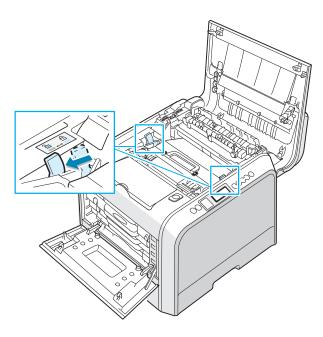
**5** Using the handle, lift the used transfer belt out of the printer by lightly pulling it towards the left of the printer.
